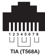
T568A Cabling Pinout Specifications
