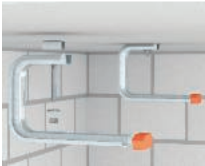
Ceiling mounting of TP wall and ceiling bracket Universal mounting of the TPD wall and ceiling bracket on the ceiling (with DS 4 spacer). Maximum tray width 300 mm.
