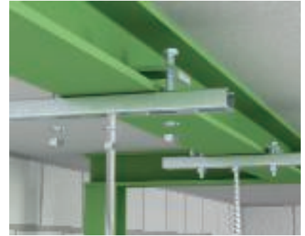
Steel clamping, C profile rail Fastening of a C profile, type CPS 4 G or CPS 5 G, to steel girder using clamping angles, type KWS.
