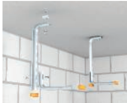
Installation of TP support with single-sided bracket fixing Ceiling mounting of a TP support with spacer DS 4 and one-sided bracket mounting. Maximum tray width 300 mm.
