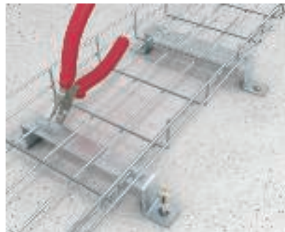
Stand-off of mesh cable trays Floor stand-off of mesh cable trays with the stand-off bracket, type DBLG 20/... Screwless fastening of the mesh cable tray on the stand-off bracket using clamping lugs.
