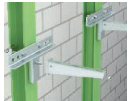
Clamp fastening on vertical steel girder Installation of the adapter plate, type KA-AW, on the vertical steel girder using clamping angle or chuck jaws. Wall brackets of type AW are fixed to the adapter plate, using the hexagonal bolt SKS 12 x 40 GF.
